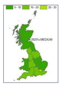
Figure 48 - Projections of the number of rail buckles (per country/region) by the 2020's with 90% level probability. Source: DEFRA (2012b).
